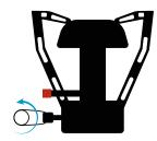
• Once the arms are in place, ignite the stove by turning the gas flow control knob ½ a turn and press the red button.
