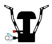
> Screw on the fuel system to the bottom of the burner.
