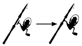
Loosen the 2 knurled nuts on the bottom of the rod. This will allow the reel collars to slide down so that the reel foot can fit into the rod seat.
